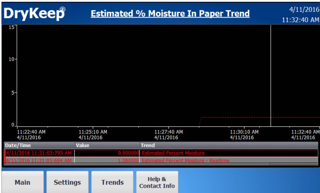
PPM and temperature values are logged every fifteen (15) minutes. Estimated percent moisture in the paper is logged once a day. All logged data can easily be downloaded to a laptop in .CSV format through the RJ45 Ethernet Panel Interface Connector mounted on the outside of the enclosure.
