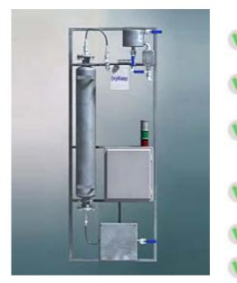
Three (3) cylinder continuous transformer dehydration and moisture monitoring system with SCADA-ready SMART controller monitoring, control, alarming, and reporting system for transformers rated 10MVA or above. System will dry the main tank oil while the transformer is in-service. Each cylinder can capture a minimum of 3, maximum of 4.2 liters of moisture before saturation and regeneration is required.
