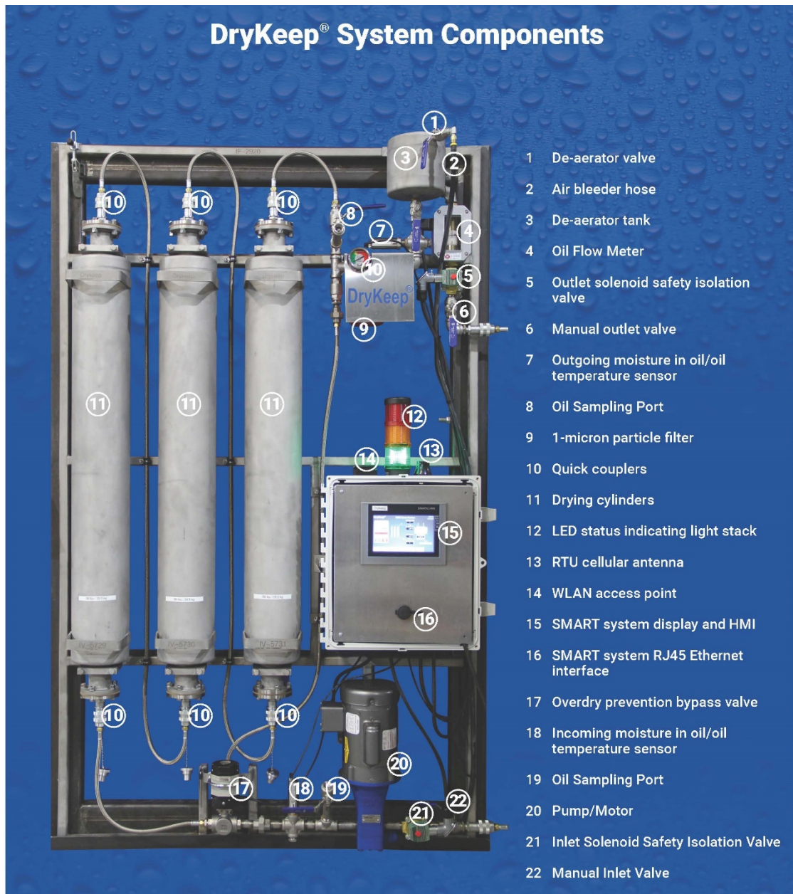
Figure 1: DryKeep® system layout
