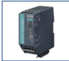
**Backup Power Supply** 24VDC UPS System with two (2) 6-cell, 12VDC, 12.0 AH, rechargeable, sealed, lead acid batteries connecting in series, 24VDC, 10 A uninterruptible power supply, battery below < 85% alarm.
