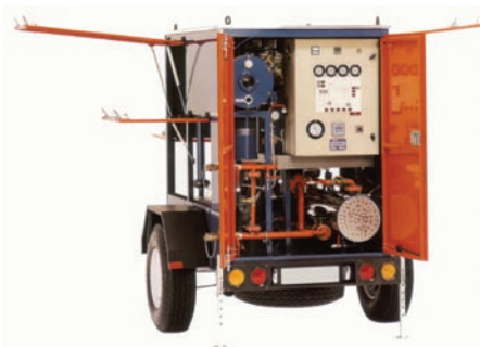
Fig. 3: Heat and vacuum moisture removal system.
